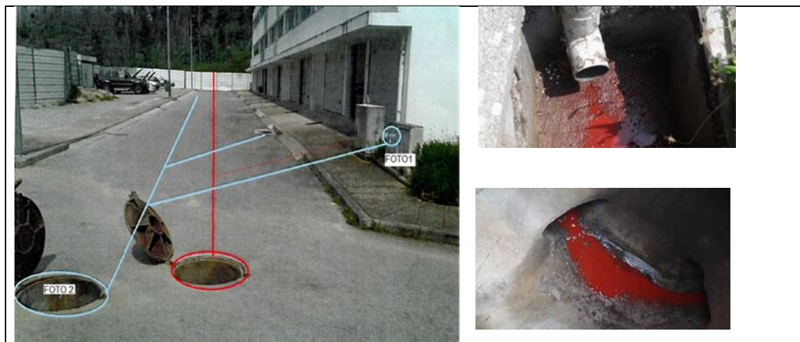
Figure 4 Monitoring drainage system (coloured effluent technique)
