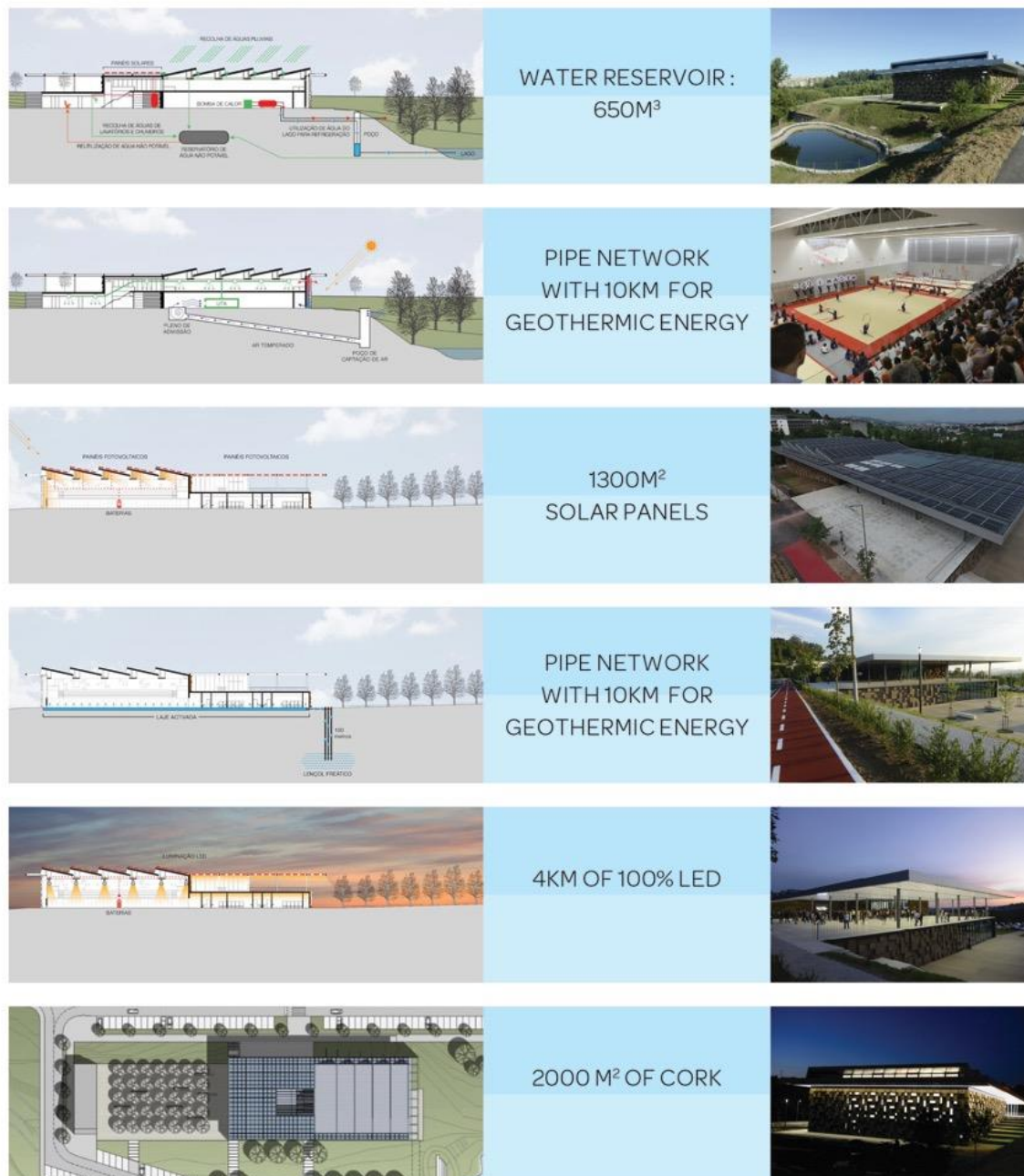
Figure 1 Gymnastics Academy, a near zero carbon building; sustainable use of soil, water, air and solar efficiency 5
